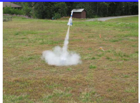
The rocket blasts off with solid fuel power and goes approximately 1,000 feet in the air. It comes down slowly, thanks to its parachute.
